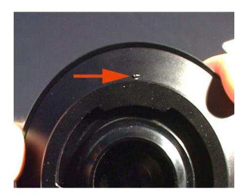
3. Now take the original BayoRing off the MK1Fisheye by turning it counterclockwise.
